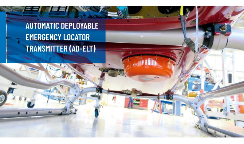
The Automatic Deployable Emergency Locator Transmitter is for operations of the helicopter over water. Increased safety by manual or automatic activation of the system. The AD-ELT system complies with EASA requirements for offshore operation of helicopters.
