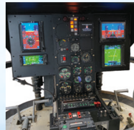
5 | Garmin G500H TXi Display of all flight-relevant information centrally in the pilot's field of view. The STC is available for Airbus BO 105. Other types upon request.
