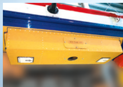
4 | Antenna bracket Antenna bracket for mounting various antennas on the tail boom of the helicopter. Mounting of different antennas on the console possible. The modification is available for Airbus types BK 117 A-1, A-3, A-4, B-1, B-2, C-1, C-2.
